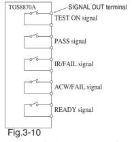
A contact which is closed when the signal is applied is called make contact, normally open contact, or form "a" contact. A contact which opens when the signal is applied is called break contact, normally closed contact, or form "b" contact. The contacts of the Tester are of the make-contact type and their rating is 125 VAC, 1 A or 30 VDC, 1 A. The withstanding voltage is 500 VAC 1 minute between the circuit and chassis.
