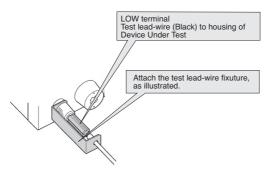
Connecting of test lead-wire on LOW side
