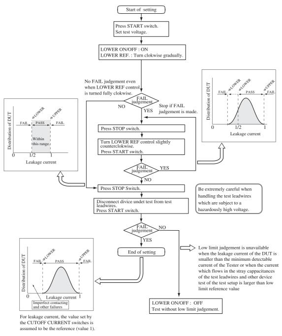
UPPER :High limit reference value of leakage current for withstanding voltage test. LOWER :Low limit reference value of leakage current for withstanding voltage test.
