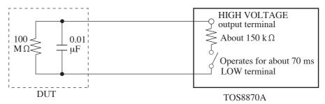
Example of discharge of equivalent circuit
